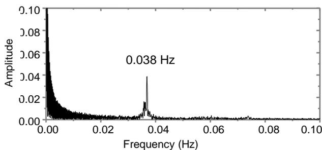
Figure 13: FFT of anode rod current fluctuations after the “dirty” AC
