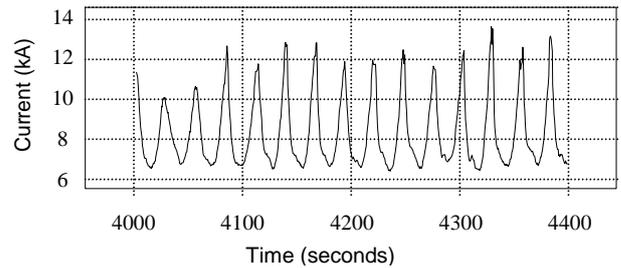
Figure 6: Fluctuation of current in anode rod 23
