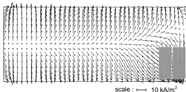
Figure 11: Current density field after the “clean” AC
