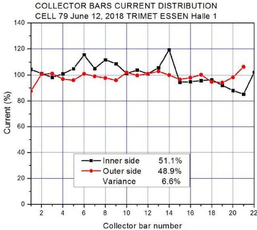
Figure 9: Current distribution with magnetic compensation
