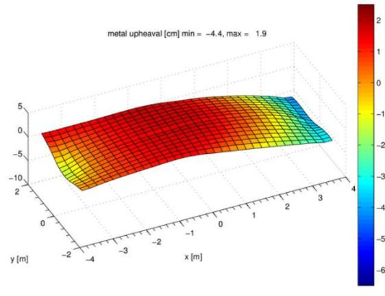
Existing busbars at 162kA, upheaval = 8.9cm      Optimized busbars at 185kA, upheaval = 6.3cm
