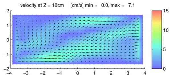
Optimized busbars at 185kA,  $v_{max} = 7.1\text{cm/s}$
