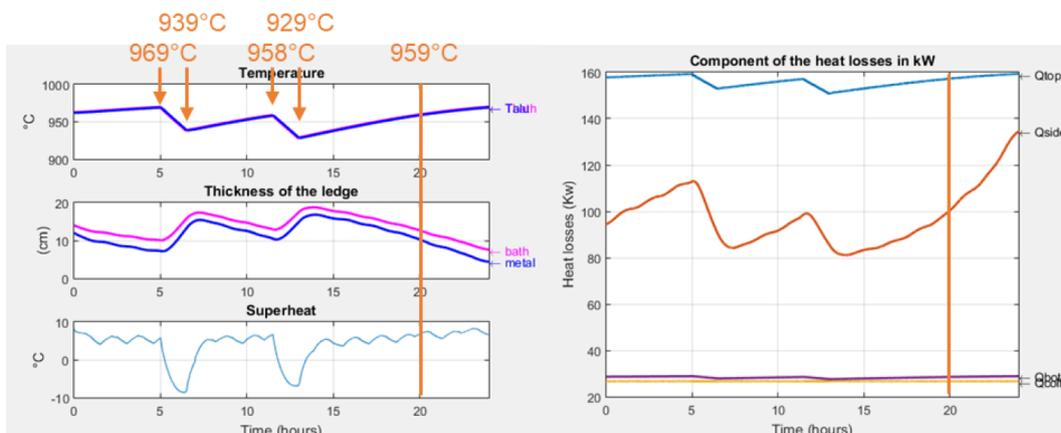
Figure 8: Cells parameters at 165 kA before, between and after the two 1.5 hours power cuts
