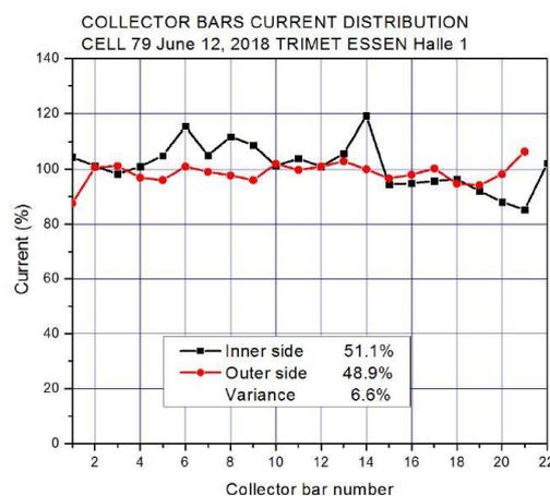
Figure 9: Current distribution with magnetic compensation
