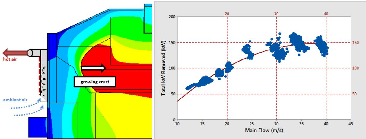
Figure 6: Schematic of Shell Heat Exchanger (SHE) Concept and the heat extraction from the booster group [6]
