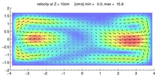
Existing busbars at 162kA,  $v_{max} = 15.8\text{cm/s}$
