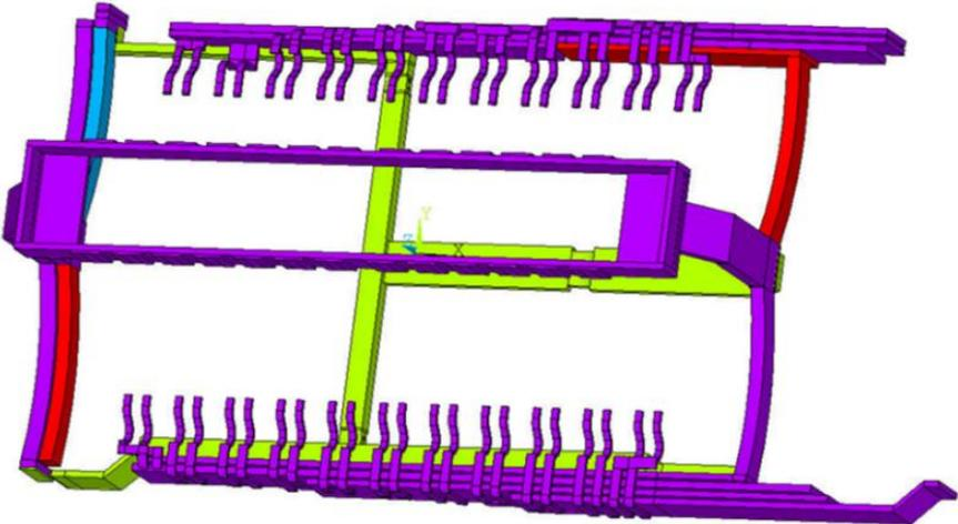
Figure 3: Optimized busbars with existing busbars in violet, new busbars in green, modified busbars in blue and disconnected or used for shortcut busbars in red
