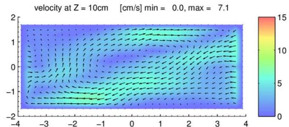
Optimized busbars at 185kA,  $v_{max} = 7.1\text{cm/s}$
