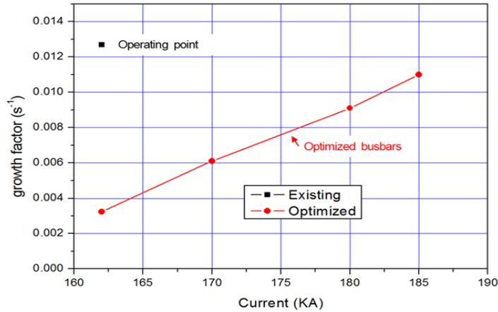
Figure 4: Maximum growth factor for the existing and optimized busbars as a function of line current (at constant internal heat generation)
