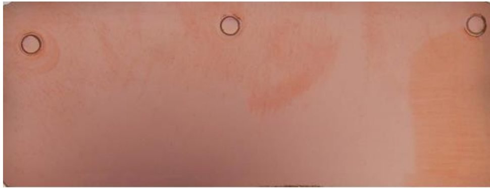
Figure 13. Copper analysis after 800 days in operation, measurement positions
