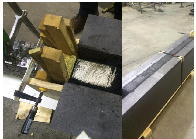
Figure 14: Block, ramming paste and electrical insulation
