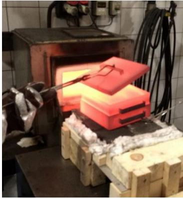
Figure 2: Box at 900°C containing the sample
