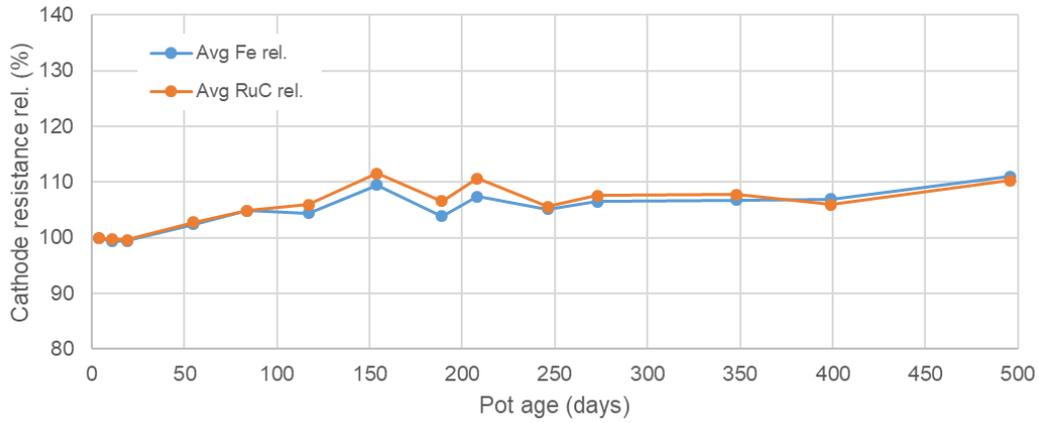
Figure 10: Relative cathode resistance for a reference cell and for RuC<sup>®</sup> cathodes
