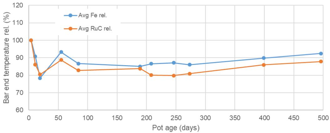
Figure 11: Evolution of the average temperature at the collector bars end
