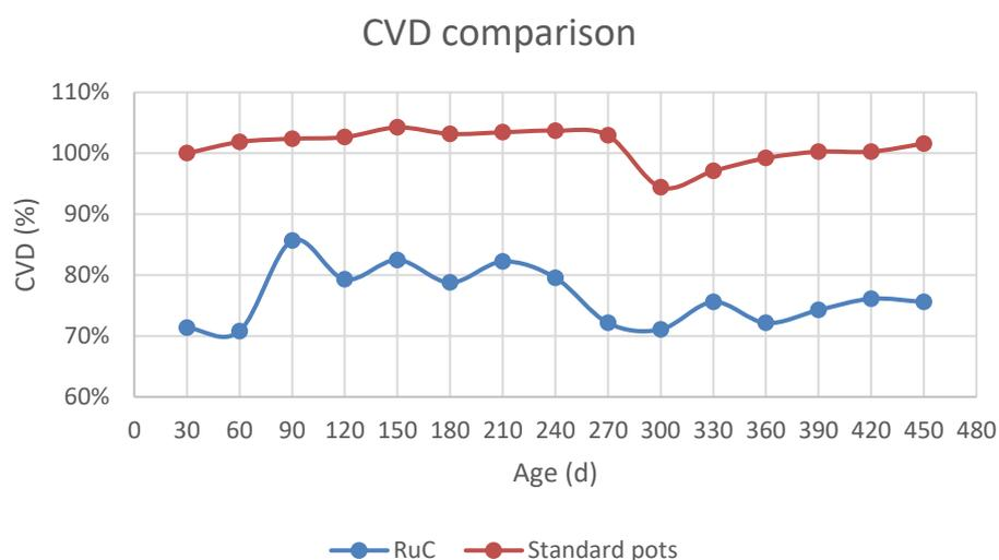
Figure 3: CVD results of RuC<sup>®</sup> cell versus reference cells after 450 days
