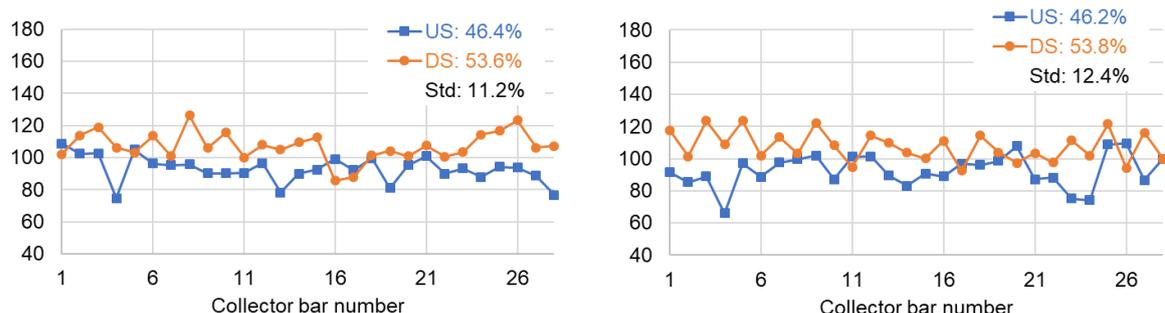
Figure 13: Collector bars nominal current distributions after 1 day and 100 days for RuC<sup>®</sup> cell
