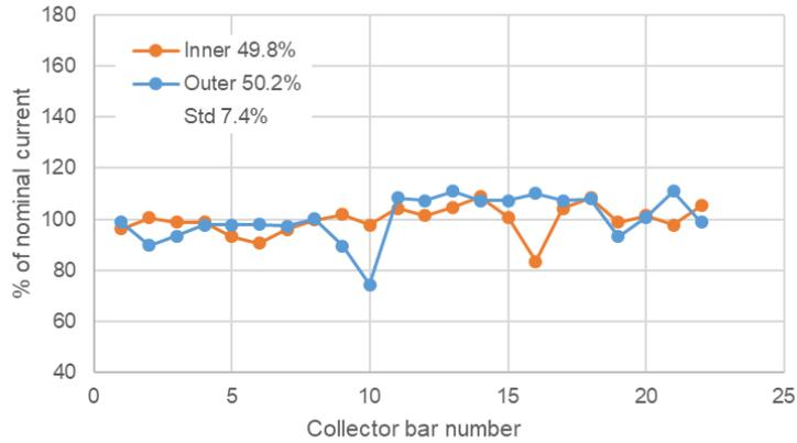
Figure 8: Collector bars current distribution after 32 days
