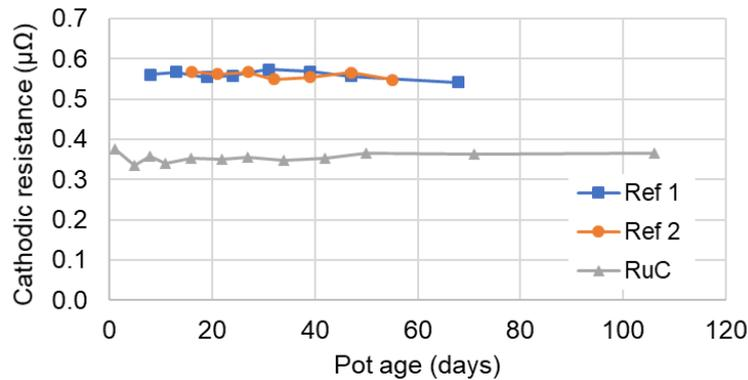
Figure 12: Cathode resistance of RuC<sup>®</sup> cell versus two reference cells (steel collector bars)
