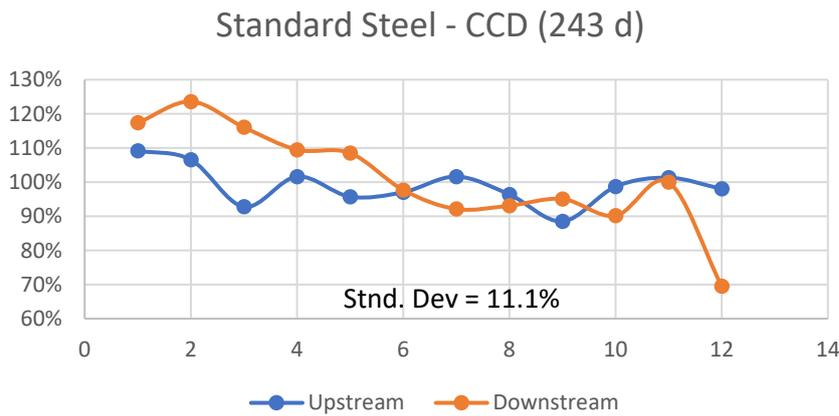
Figure 5: CCD of a reference cell after 243 days
