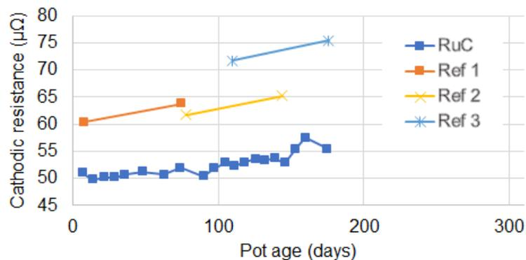
Figure 7: Cathode resistance for reference cells and for a RuC® cell
