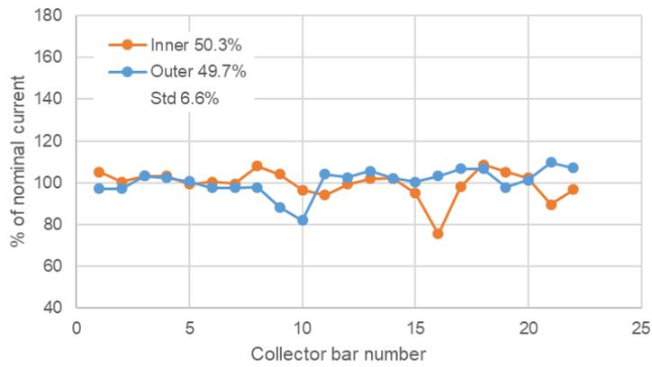
Figure 9: Collector bars current distribution after 154 days
