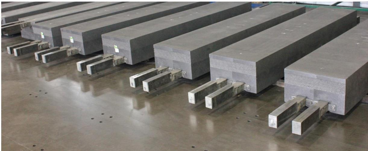
Figure 2: RuC<sup>®</sup> cathodes ready to be shipped
