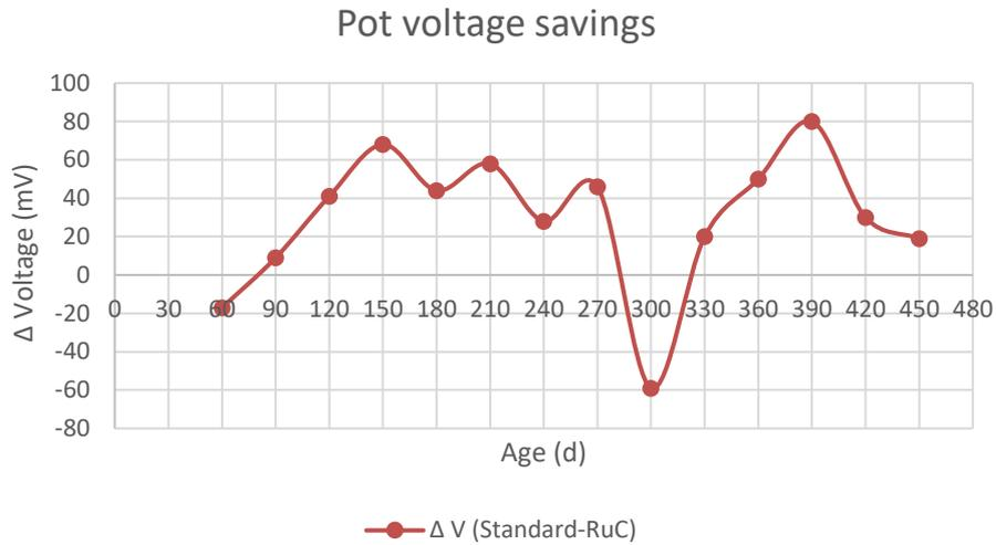
Figure 4: Cell voltage savings of RuC<sup>®</sup> cell versus reference cells during first 450 days of operation
